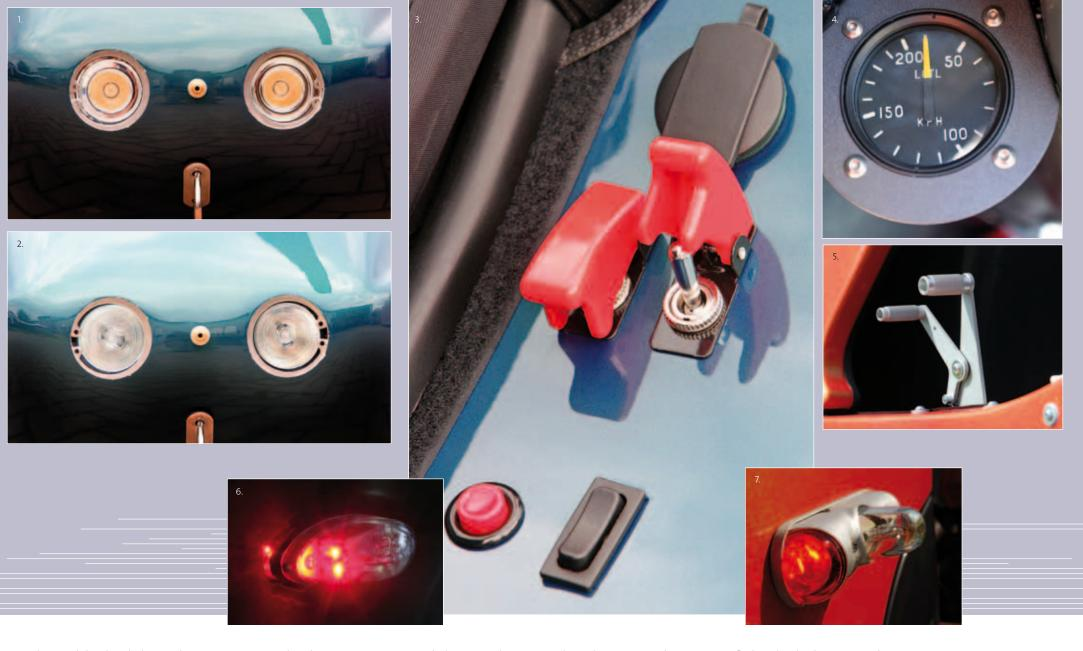
Pilots with landing lights are better seen in air and in the approach – the halogen bulbs (2) are 2 x 50W, the LED lamps (1)  $2 \times 2.5$  W.
