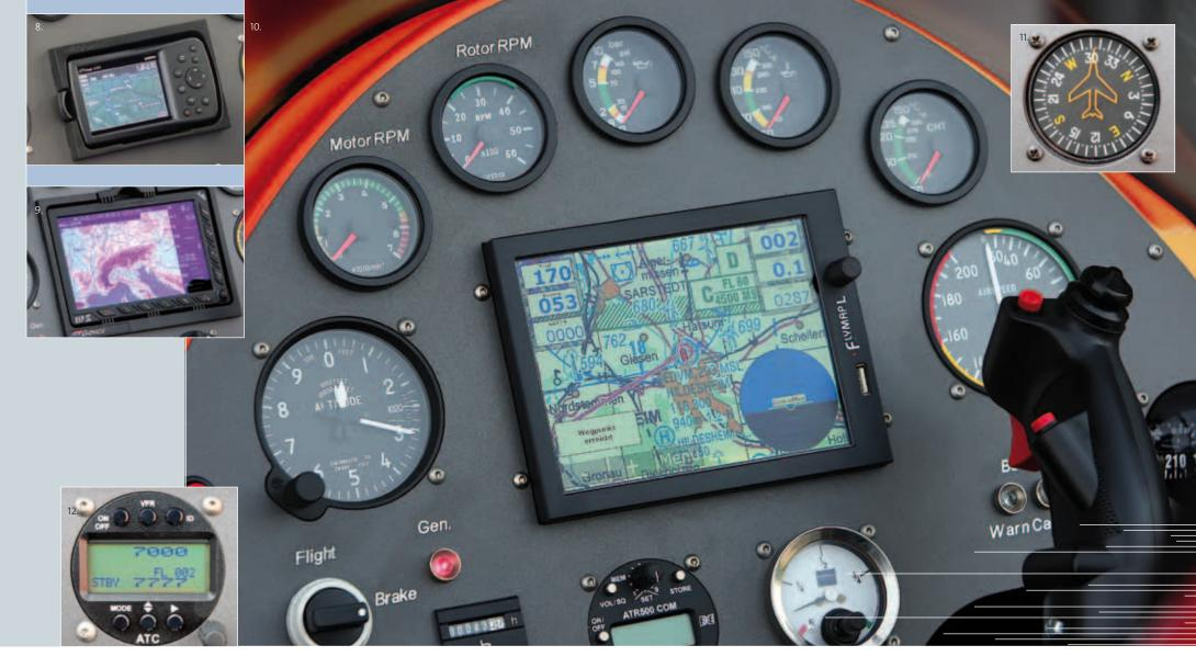
Clearly arranged and visually correct, the GPS cockpit panel permits the integration of the following GPS devices: FlyMap L (10), GPS MAP 196/296/396/495/496 (8) as well as AvMap EKP IV color (9). The standard instrument panel includes (from left) hour meter, altimeters, engine and rotor speed, oil pressure, oil temperature, cylinder head temperature, airspeed indicator, ball compass.
