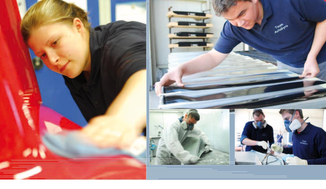
Composite GRP components (glass or carbon fibre) are created in our in-house developed and manufactured moulds, and painted in our own high class paint shop.
