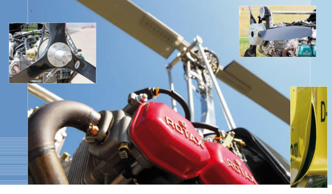
The MTOsport is propelled by a Rotax engine. This extremely reliable 4 cylinder is offered in two variants: 914 UL turbo with 115 HP or 912 ULS with 100 HP. As an option the 912ULS can be fitted with an airbox. The optional air scoops (4), whilst
