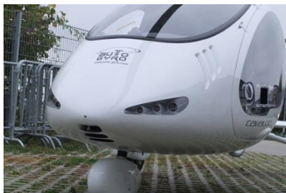
Air intake and gills for condenser
